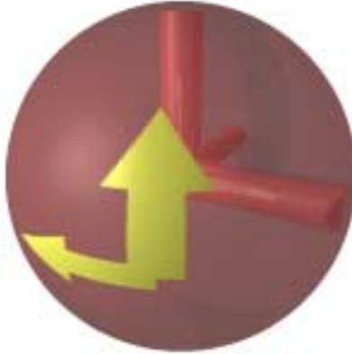
Figure 4 – A representation of the camera’s spherical motion. The arrows point in the direction of positive rotation.
